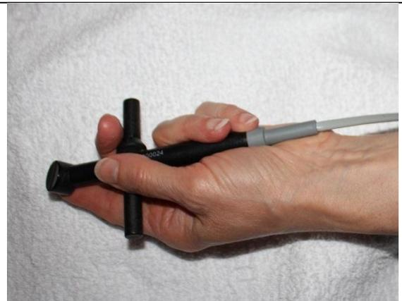
Figure 2; Single Crystal Ultrasound Transducer, note grip required.
